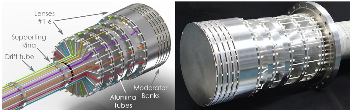
Fig. 3.3.5 - A 3-D model and a picture of the constructed new generation Platinum based positron source
