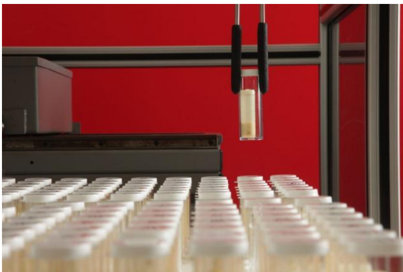
Fig. 3.6.1 – Automated NAA Sample Analyzer
