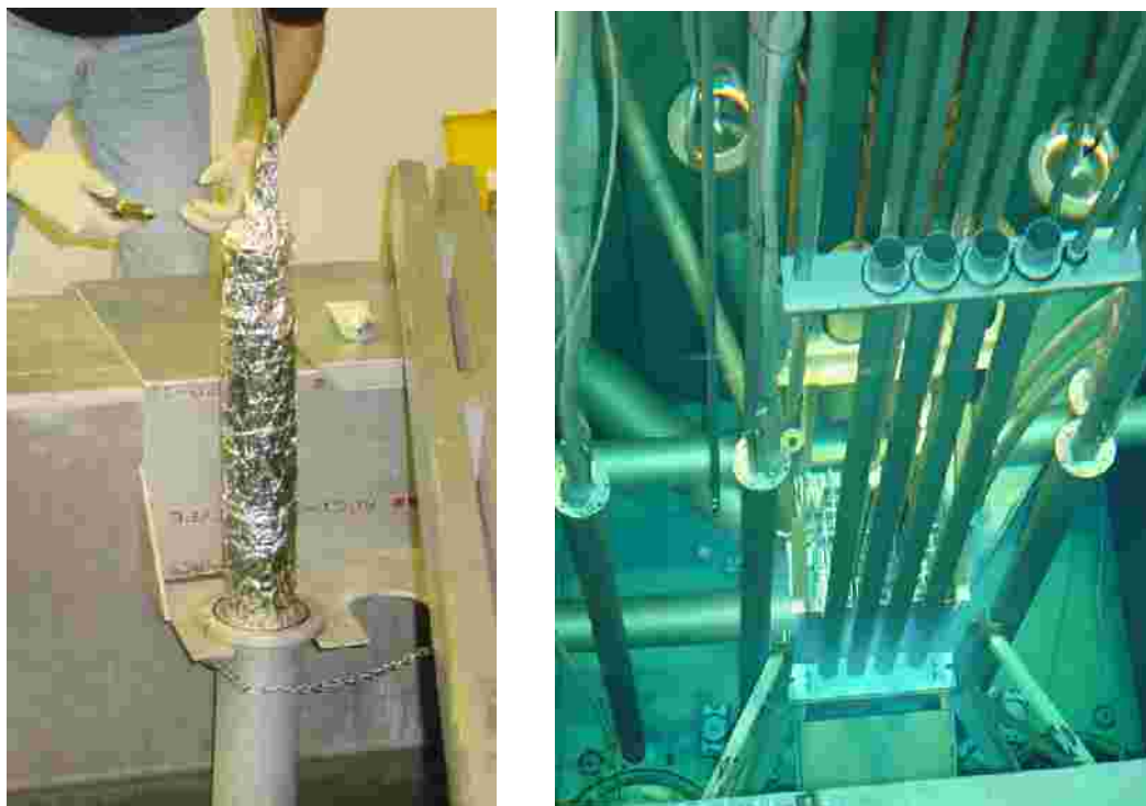
Fig. 3.7.3 – Irradiation Testing of Ex-Core Neutron Detectors to 1\text{E}18 NVT Thermal Fluence in 3500 MW-hrs exposure. 3.5" ID Standpipes utilized (at right).
